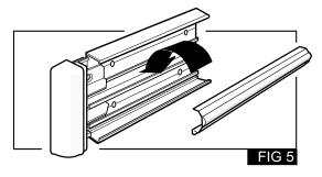
Avoid joints in aluminium and Impact Absorber coinciding.
